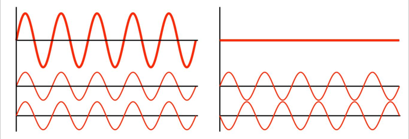
This shows the constructive and deconstructive superposition of two waves (the thick line is the final wave).
